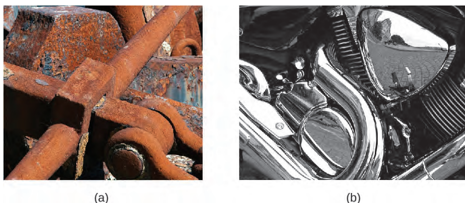
Figure 1.19 (a) One of the chemical properties of iron is that it rusts; (b) one of the chemical properties of chromium is that it does not. (credit a: modification of work by Tony Hisgett; credit b: modification of work by "Atoma"/Wikimedia Commons)
