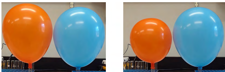
Figure 9.29 The left photograph shows two balloons inflated with different gases, helium (orange) and argon (blue). The right-side photograph shows the balloons approximately 12 hours after being filled, at which time the helium balloon has become noticeably more deflated than the argon balloon, due to the greater effusion rate of the lighter helium gas. (credit: modification of work by Paul Flowers)
