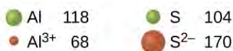
Figure 6.32 The radius for a cation is smaller than the parent atom (Al), due to the lost electrons; the radius for an anion is larger than the parent (S), due to the gained electrons.
