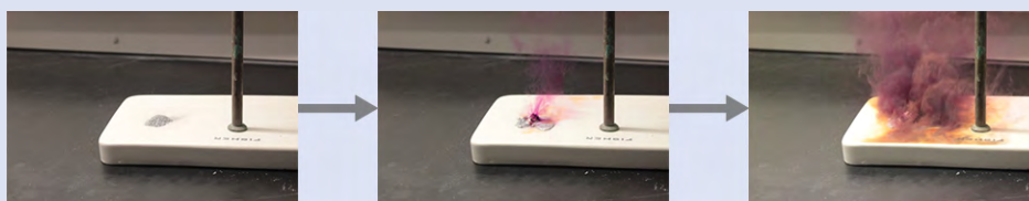
Figure 4.10 Aluminum and iodine react to produce aluminum iodide. The heat of the reaction vaporizes some of the solid iodine as a purple vapor. (credit: modification of work by Mark Ott)
