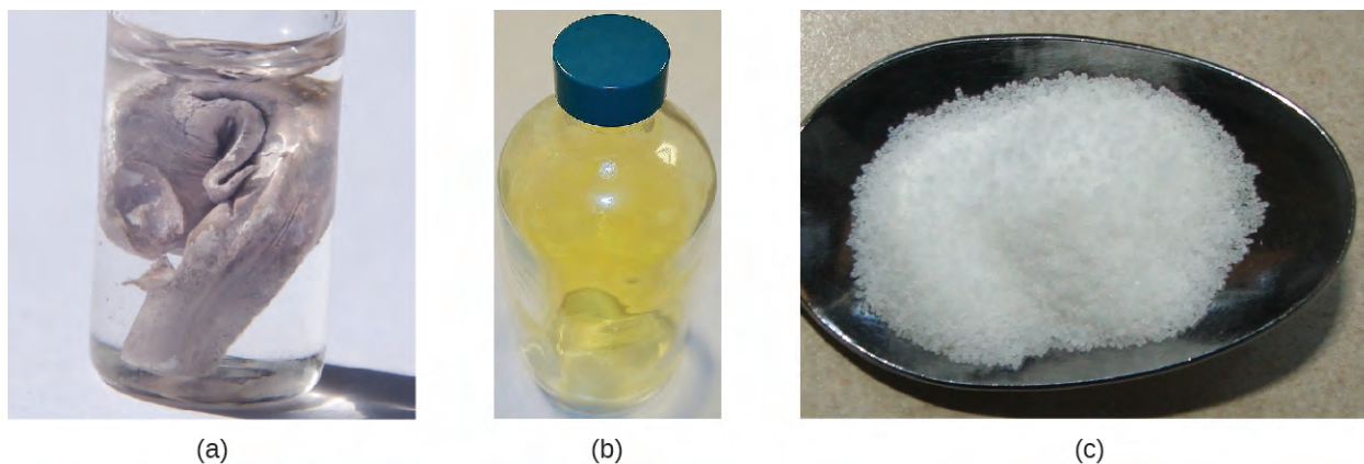
Figure 7.2 (a) Sodium is a soft metal that must be stored in mineral oil to prevent reaction with air or water. (b) Chlorine is a pale yellow-green gas. (c) When combined, they form white crystals of sodium chloride (table salt). (credit a: modification of work by “Jurii”/Wikimedia Commons)
